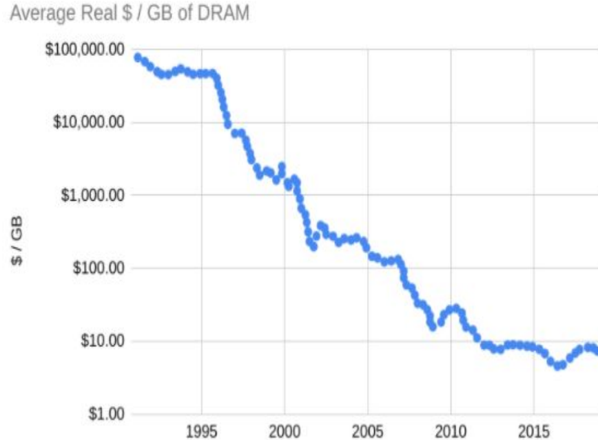
Figure 2: Average $ / GB of DRAM from 1991 to 2019 according to Objective Analysis. Dollars are 2020 dollars.
